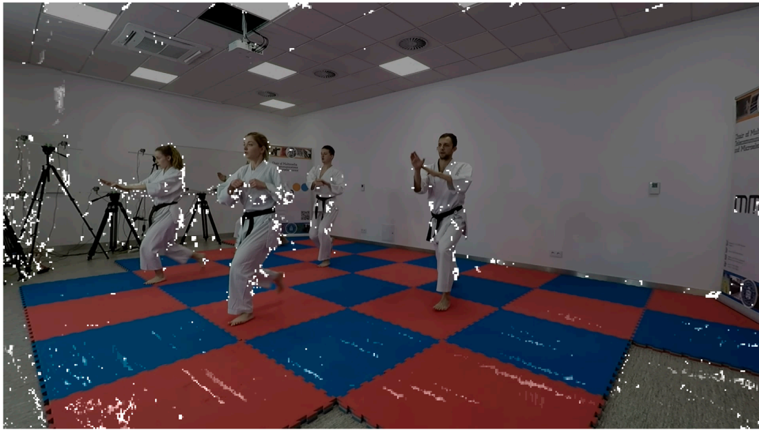
Figure 4. The visualization of differences in depth maps estimated using alpha-expansion and the proposal. Areas estimated differently (shown as white areas) are overlaid on input view.
