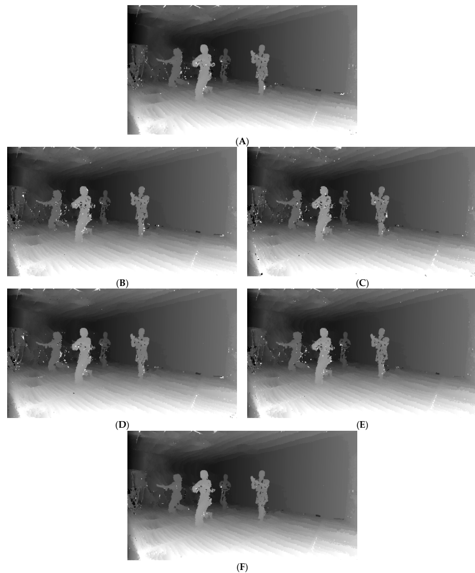
Figure 3. The comparison of depth maps estimated for the MartialArts sequence. Depth maps estimated using graph-cut optimization with: (A) alpha-expansion, (B) hierarchical alpha-expansion ( n = 2 ), (C) hierarchical alpha-expansion ( n = 4 ), (D) hierarchical alpha-expansion with second-cycle label shift ( n = 2 ), (E) hierarchical alpha-expansion with second-cycle label shift ( n = 4 ), (F) hierarchical alpha-expansion with second-cycle label shift and neighboring segments label examination.
