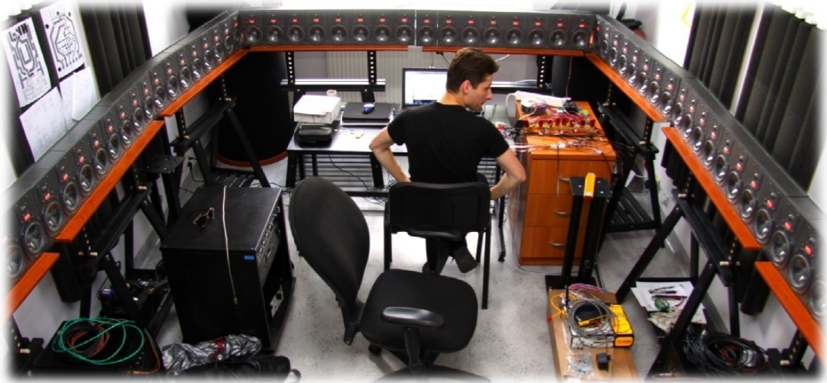
Fig. 2. Experimental WFS system at the Poznań University of Technology
