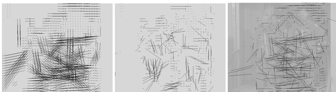
Fig. 5.38. Interpolated motion vectors estimated for resolution 352 \times 288 , motion vectors estimated for resolution 704 \times 576 and differential motion vectors in the frame with the highest value of parameter \overline{\Delta mv_{HL}} ( \overline{\Delta mv_{HL}} = 159.053 , \overline{\sigma_{HL}} = 248.309 ). Frame number 63 from Crew sequence, Q_P = 41 .
