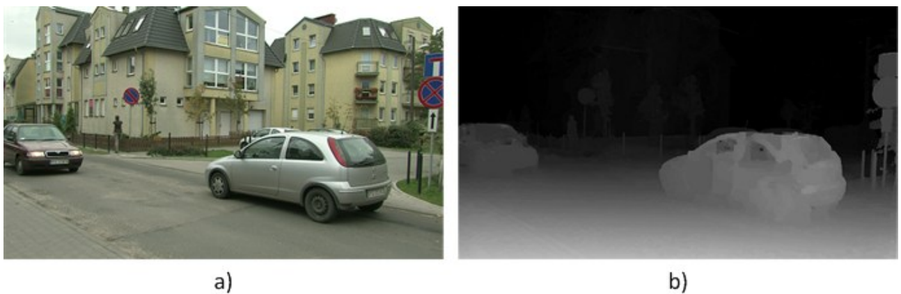
Fig. 1.1. An example of: a) texture and b) depth from 3D video test sequence Poznan Street .
