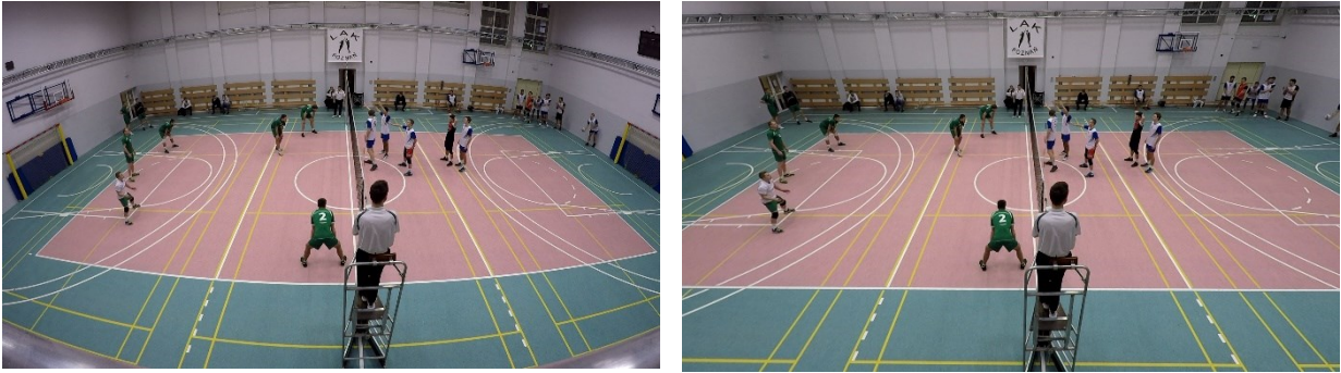
Fig. 4. One frame from a volleyball match sequence: before lens distortion removal (left) and after lens distortion removal (right).
