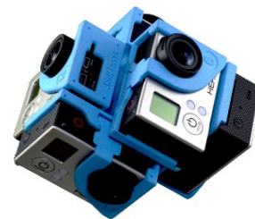
Fig. 4. 360-degree camera built from six GoPro Hero 3 action cameras (photo by the authors).
