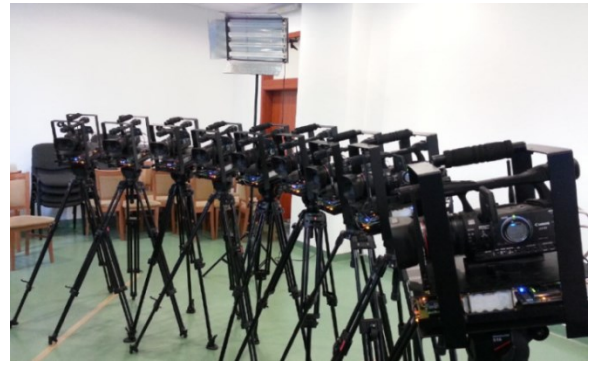
Fig. 9. Experimental free viewpoint acquisition system built at Poznan University of Technology.
