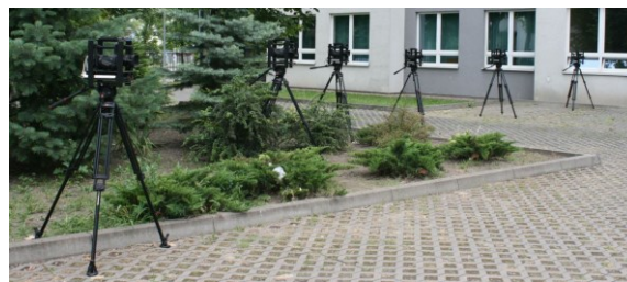
Fig. 3. Wireless multi-camera system for FTV test video capture
