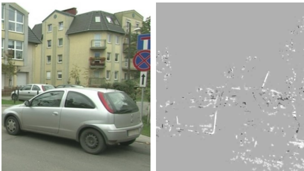
Figure 4. Noise reduction with MCNRR technique - the filtered frame of “Poznan Street” sequence (left) and difference between the denoised frame and the original one. Gray level represents zero value (no difference)
