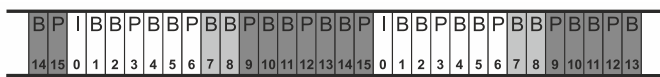
Figure 2. The location of watermarked and non-watermarked frames in watermarked video sequence. The frames marked in dark are watermarked (from [2]).
