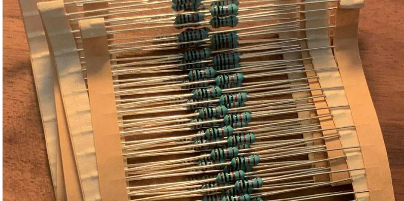
Figure 5.4 Presents Resistors 10kΩ with 1% Tolerance used for audio measurement project (Personal Photo)
