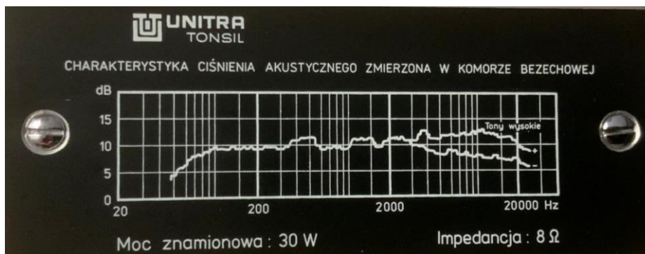
Figure 3.3 Acoustic Pressure Characteristics Measured in an Anechoic Chamber Unitra Tonsil ZG-30-C115. (Personal Collection).
