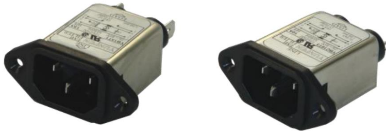
Figure 7.11 Presents an AC supply socket with filter (3A, 250VAC), model FYB03T1 produced by YUNPEN ELECTRONIC. As stated in manufacturers documentation, [42], “General purpose filter with IEC connector providing effective line-to-ground noise up to 15 amp”.
