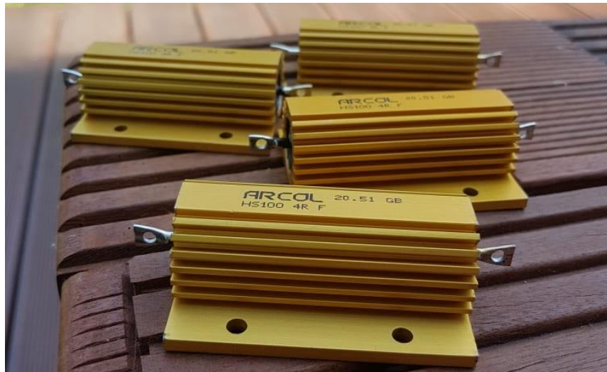
Figure 5.3 Resistors 100W 4 Ohm 1% Tolerance used for Audio Measurements (Personal Photo)
