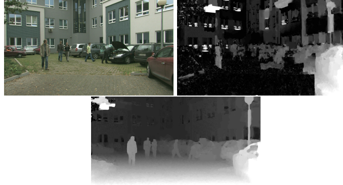
Fig. 3. Image of the scene (top left), depth map estimated for test sequence without rectification (top right) where significant artefacts can be seen and after rectification with proposed algorithm (bottom) with very limited amount of artefacts.
