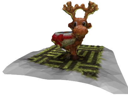
Fig. 5. Example of reconstructed surface from point cloud.
